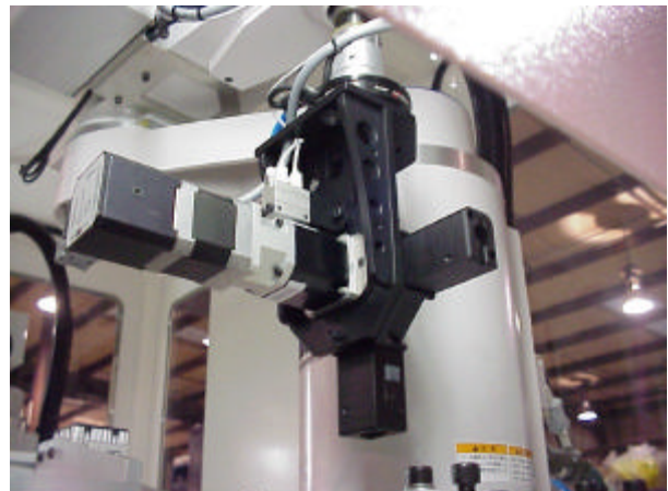
Servo Driven Gripper Turret Accommodates Different Component Types
